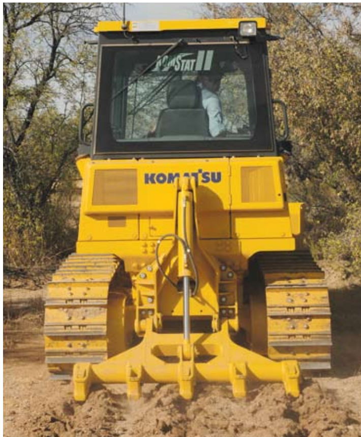
Falcon Valley equipped its Komatsu D39EX-21 dozer with a ripper for turning up hard soils. "It's very versatile which is a major plus," Grant Wilson said of the machine. "I use it for ditching when we run new water lines by turning the blade sideways and at an angle. It works really well."
