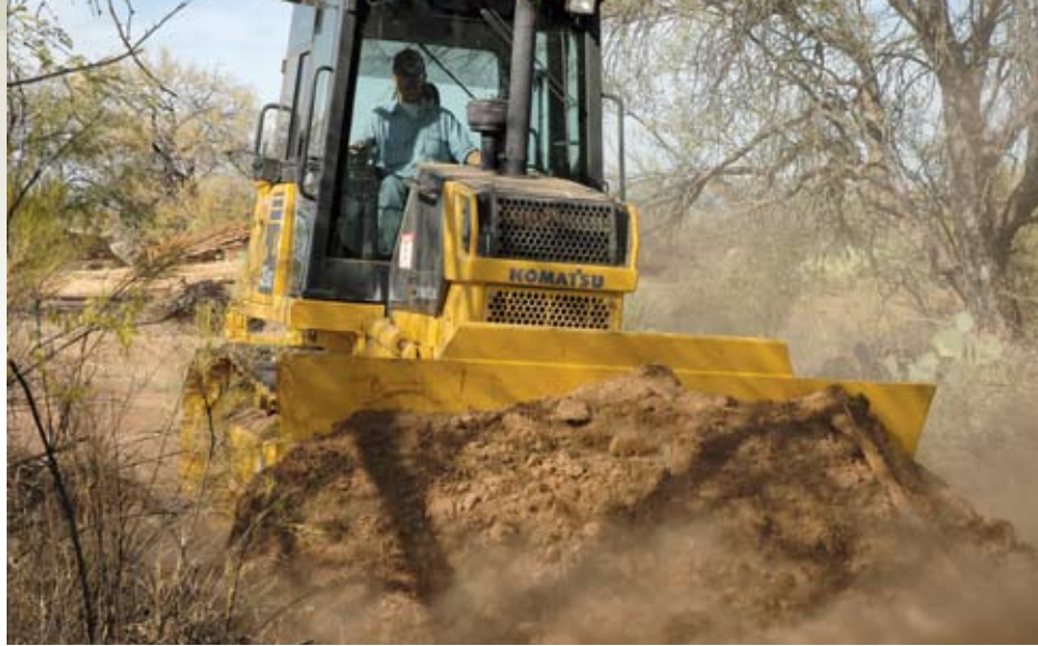
Grant Wilson uses Falcon Valley's Komatsu D39EX-21 Komstat II dozer to push material at the 64,000-acre ranch. The 95-horsepower machine is used for road building and repair, pond construction and cleaning, as well as a variety of other tasks. "It's been a real time-saver," said Wilson. "Jobs that used to take two weeks with our old equipment can now be done in a couple days."
