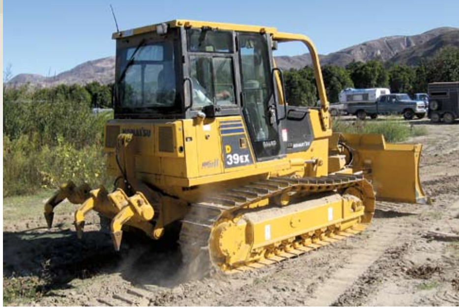
Bryan Hedrick just took delivery of this brand-new Komatsu D39EX-21 dozer. "I really like the pressurized cab because I often work in very dusty conditions," he noted.
