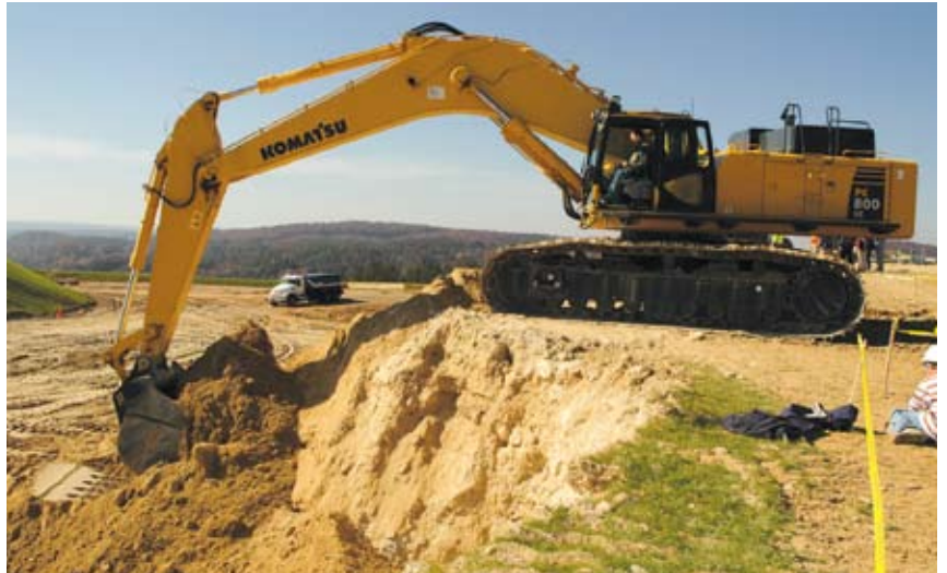
The 956-horsepower PC2000-8 (above) is a new machine that replaces the PC1800 in the Komatsu excavator lineup. Similarly, the new PC800LC-8 (below), has more horsepower and greater stability than the PC750 it replaces.
