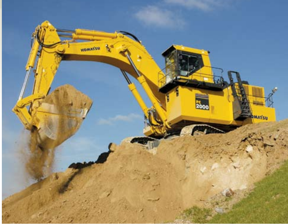
The 956-horsepower PC2000-8 (above) is a new machine that replaces the PC1800 in the Komatsu excavator lineup. Similarly, the new PC800LC-8 (below), has more horsepower and greater stability than the PC750 it replaces.
