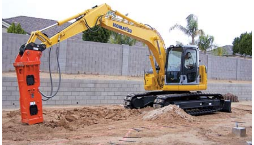
A Dirt Artist operator uses the company's PC138USLC-2 excavator to dig a new pool in the Phoenix area. The company equips its five Komatsu excavators with quick couplers to easily switch from buckets to NPK hammers it uses for demolition and breaking through rocky soils. "I've been a Komatsu man from day one," said Owner and President Jason Shawd. "They have tremendous power, and they're fast. The breakout force and cycle times are much better compared to other brands of equipment we've tried."
