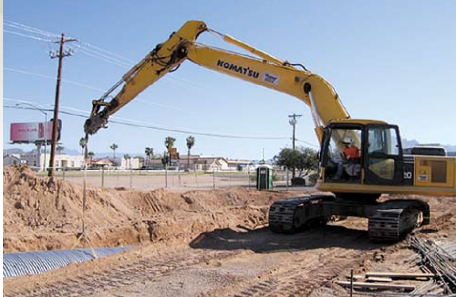
Setting pipe is one of several tasks for which Code One Construction uses its Komatsu PC220LC-7 excavator. The company also digs trenches and compacts with the 53,350-pound machine.
