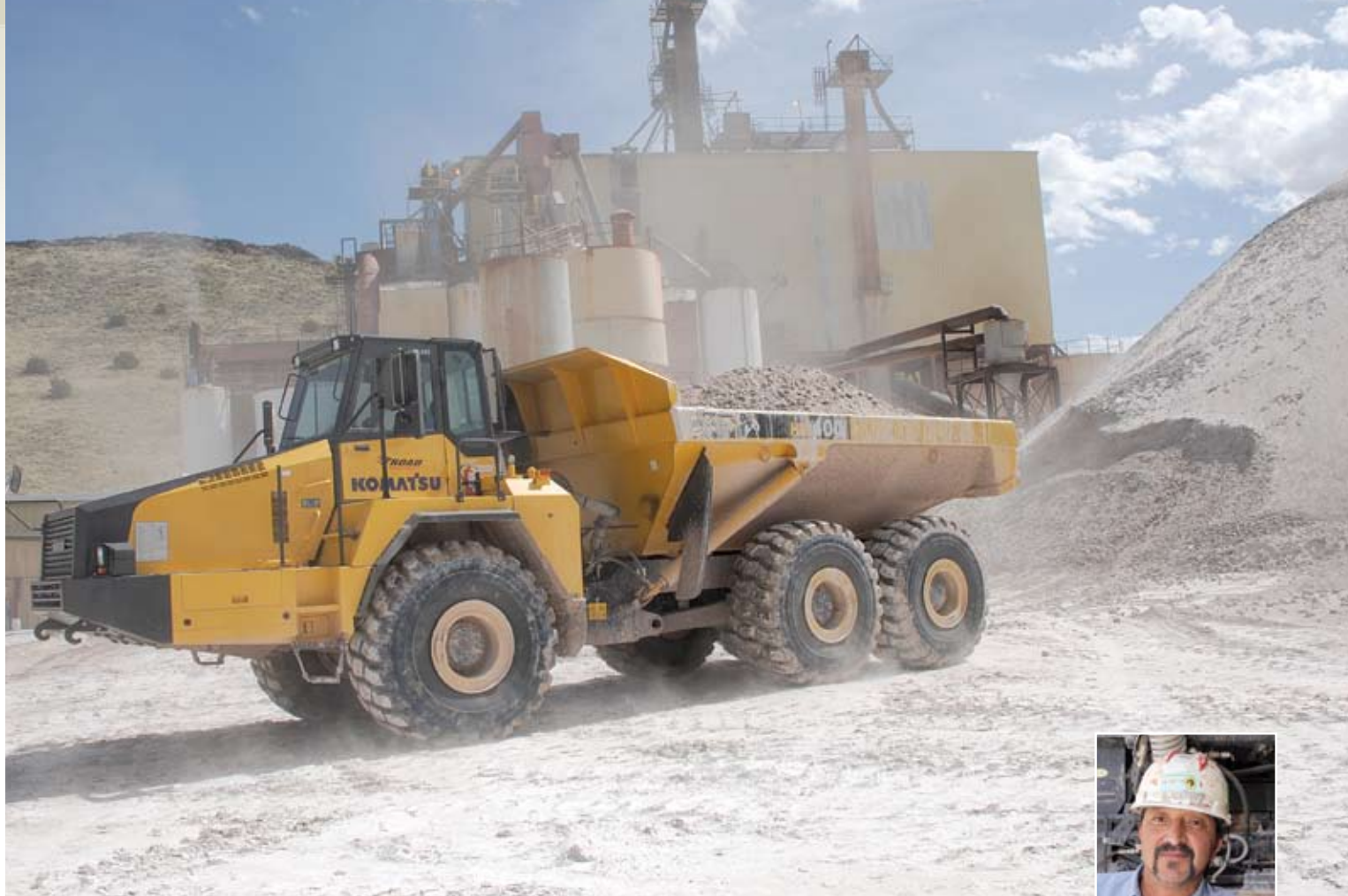
Using a Komatsu HM400 articulated dump truck, Driver Joe Lopez brings a load of perlite to the crusher at the Dicaperl Minerals Socorro Plant in Socorro, N.M. "It really has good climbing ability, horsepower and maneuverability," said Lopez.
