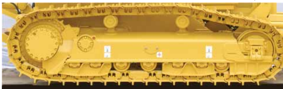
Komatsu's PLUS undercarriage system as much as doubles the life of a crawler track compared to conventional types used in both sand and clay.
