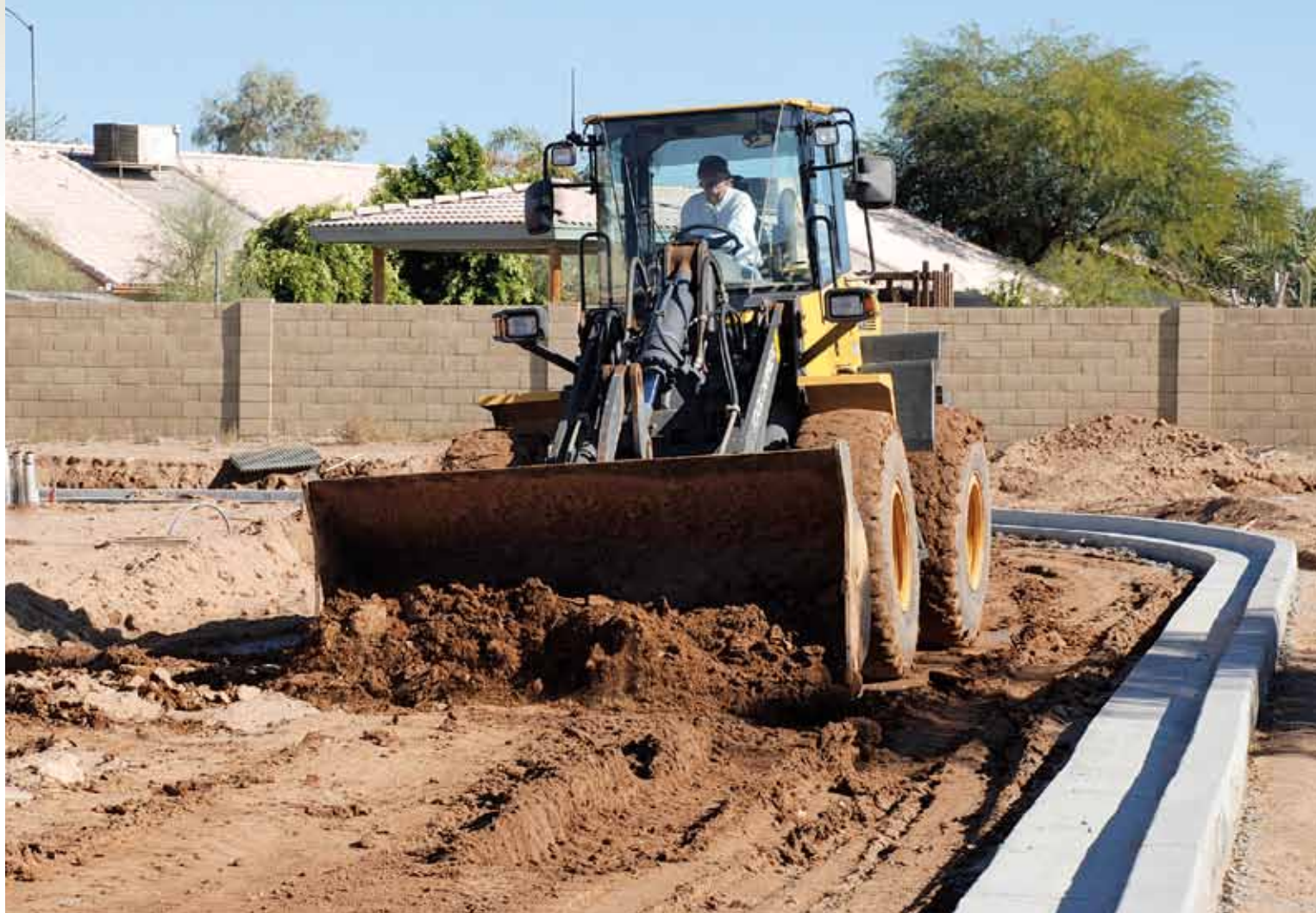
JWJ Pipeline & Excavation uses its WA250-5 parallel tool carrier for grading, backfilling and hauling pipe.
