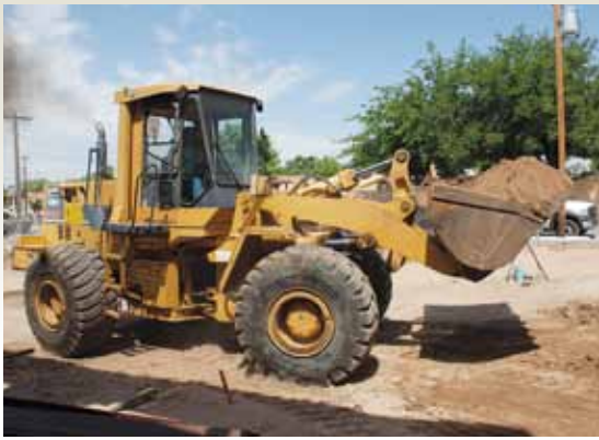
Groundhog Excavating uses this WA380 wheel loader for cleanup and load-out on its demolition projects.
