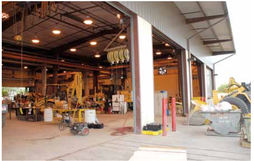
The shop area features eight deep service bays that can each accommodate two machines at once, as well as two 10-ton overhead cranes.
