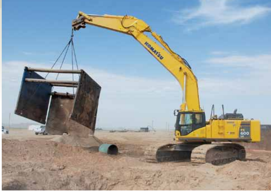
A Petra Contracting operator lifts a trench box with a PC600LC-8 the company recently rented from Road Machinery, LLC. "The Komatsus are stronger, and at the same time more fuel-efficient than our other brand," said Owner/President Keith Riefkohl. "They also come with some features, such as KOMTRAX, that aren't standard on other brands. Komatsu is definitely our brand of choice now."
