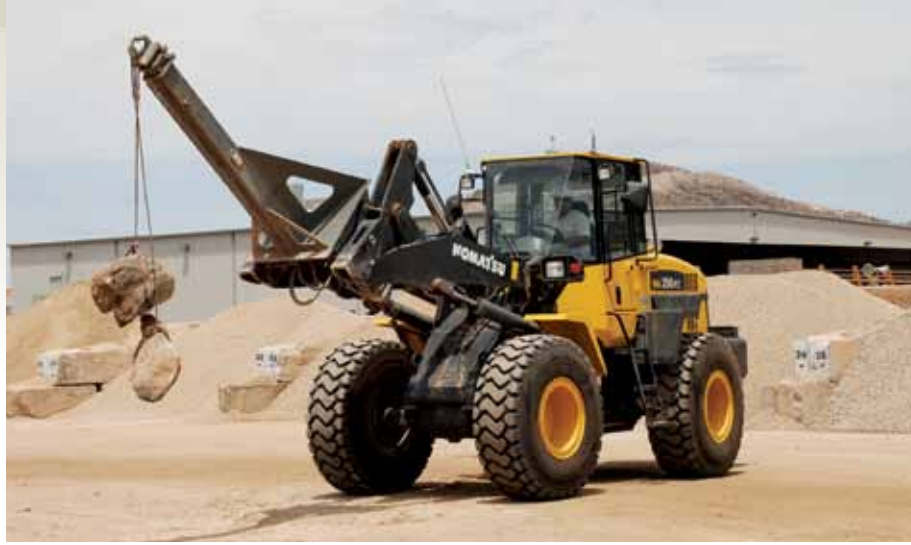
Pioneer Landscaping Materials likes the versatility its Komatsu parallel tool carriers offer. This WA250PZ-6 has a quick coupler for fast attachment changes from its specialty attachment for carrying boulders to a bucket for load-and-carry applications.
