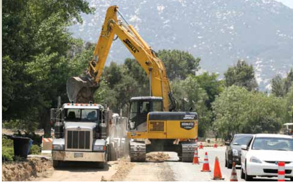
Recent acquisitions include a Komatsu PC228USLC tight-tail-swing excavator. "The PC228 is a huge hit with our customers," said Erin Oskorus, Savala Equipment Rentals' CEO. "It can get into tight areas or work in a traffic lane without the worry of the back end swinging around and hitting something."
