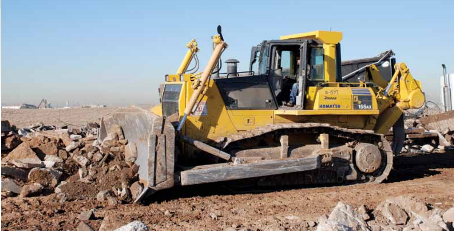
Using a Komatsu D155AX dozer, a Breinholt Contracting operator pushes construction debris at the company's landfill in southwest Phoenix.
