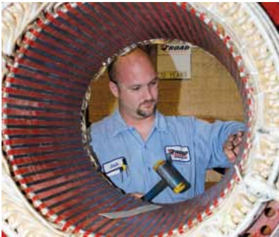
Josh Greener works on a truck stator at the Phoenix shop.
