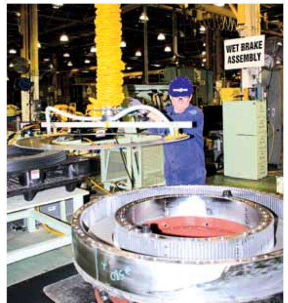
Quality components make up the truck, including the wet-disc brakes which are assembled at PMO.
