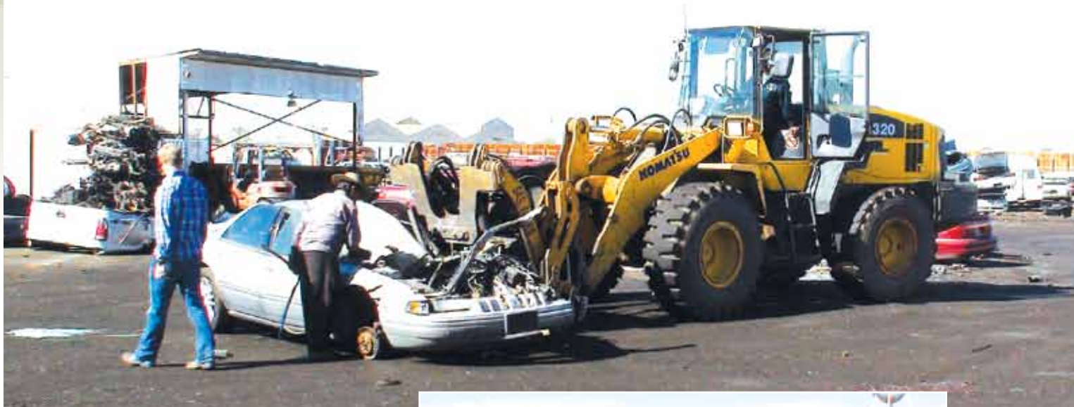
Arizona Auto Parts and its subsidiary, Pull-N-Save, get versatility from their Komatsu loaders, especially its WA250PZ-6 (right) that's used to move autos and its WA320 (above), which uses a specialty "Scorpion" attachment to pull engines and transmissions before a car is crushed.
