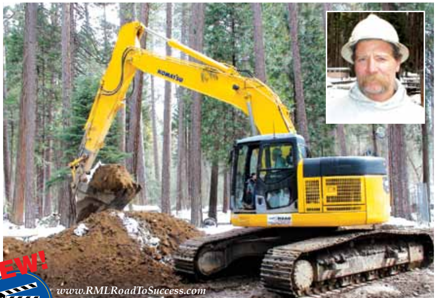
Operator Randy Foley uses a Komatsu PC308USLC excavator to dig on a project in Yosemite National Park. "The tight tail swing of the PC308 is a real advantage for projects like this one where we're basically in the middle of the woods," said Justin Allison. "We can dig and move material without worrying about hitting trees. It's very productive."
