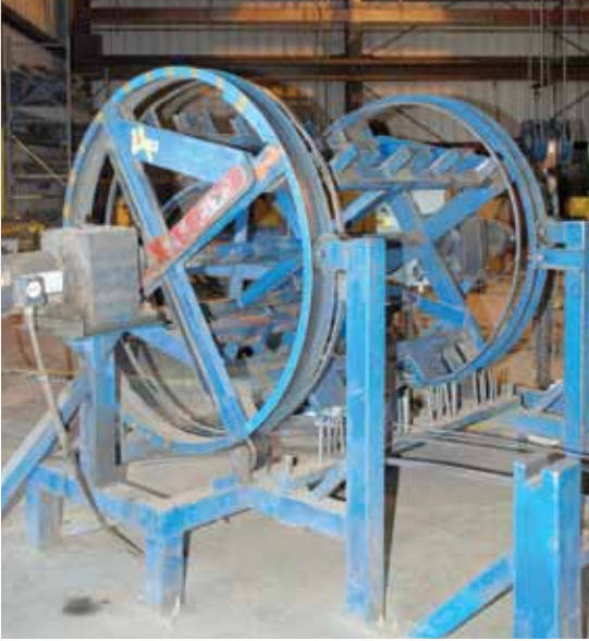
Road Machinery's Tucson Hydraulic Reman shop continues to fabricate specialty items for CXT, such as this reel used to hold prestressed wire strands that are used in manufacturing concrete railroad ties.
