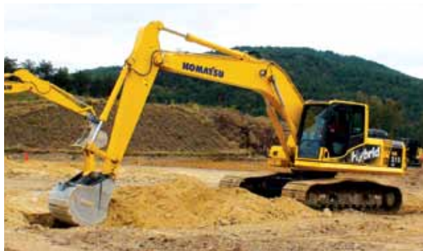
Among the machines at Demo Days was the Komatsu HB215LC-1, the world's first and only hybrid excavator.
