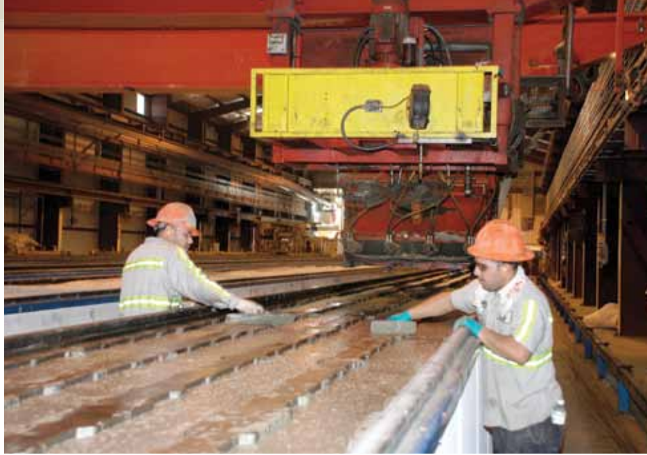
As concrete is poured into forms, CXT workers smooth it out.
