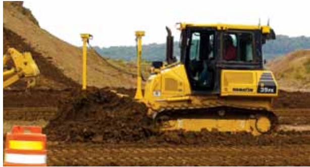
Operators could experiment with several dozers at Demo Days, including this low-ground-pressure D39PX-22, equipped with a 3D machine-control system.
