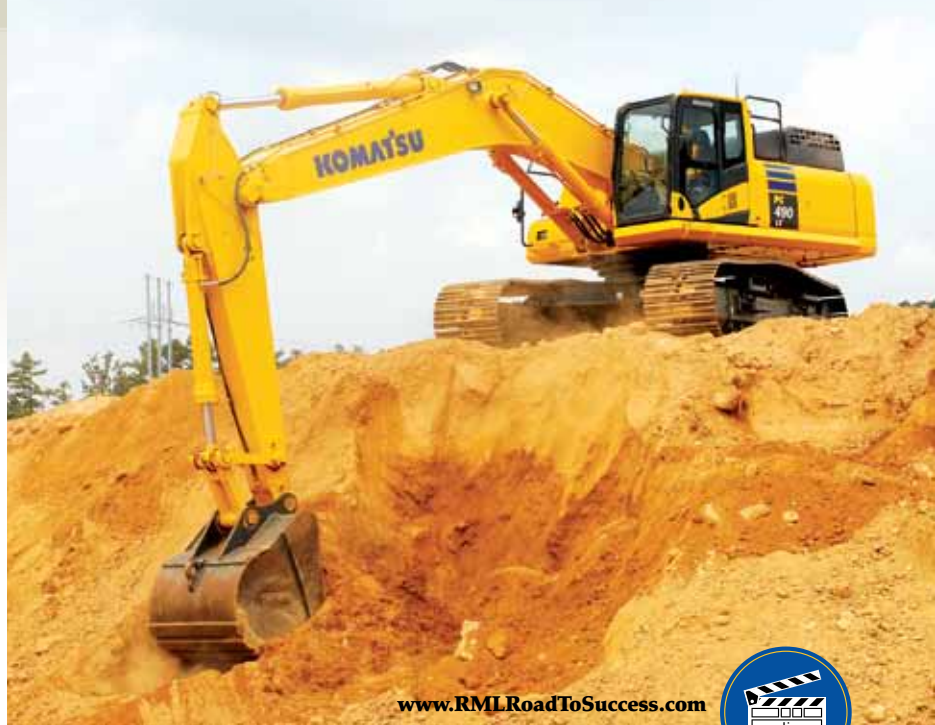
The 360-horsepower Tier 4 Interim PC490LC-10 is the largest excavator produced at Komatsu's Chattanooga Manufacturing Operation. The facility also manufactures four other Tier 4 Interim excavators, as well as the PC200LC-8.
