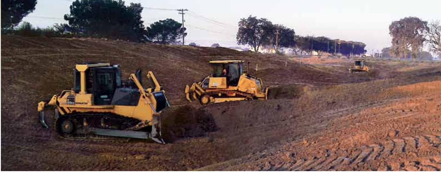
Diamond D General Engineering owns several Komatsu dozers, including a D65EX-15, a new Tier 4 Interim D61EX-23 and a D51EX-22, all shown here working together at a job in Woodland, Calif. "We started using Komatsu dozers because I believe Komatsu's quality and technology is now far superior to the brand we were running," said Owner/President Spencer Defty.
