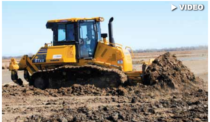
The most recent addition to Diamond D's fleet is this Komatsu D61EX-23 dozer, used here to grade dirt on a farm project near Woodland, Calif. "I believe the new D61 is really in a class by itself. With its production ratio and the power-angle-tilt blade, it has the capacity to do large cut/fill projects, while at the same time being nimble and agile enough for finish work," said Owner/President Spencer Defty.
