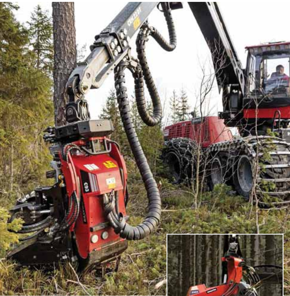
New C-Series “carry style” harvesting heads feature Komatsu’s Constant Cut™ saw control system with a saw bar that includes a 19cc saw motor with an integrated valve to deliver precise control of hydraulic flow and pressure. MaxiXplorer™ 3.1 is also standard and a complete system for machine control, head control, cross cutting and administration.
