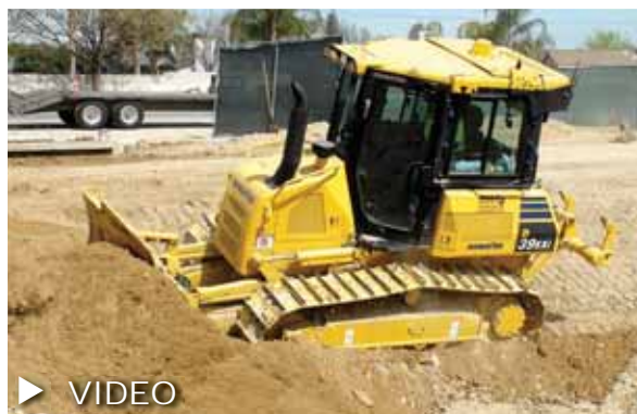
Ground Breakers Construction has rented Komatsu intelligent Machine Control dozers, including this D39EXi-23 it used on a project in Bakersfield. "The dozers save us time and money because they are accurate and keep us from overcutting," said General Foreman Milford Martin.
