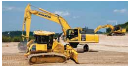
Attendees could operate all equipment, including the D155AXi-8 RC dozer, which is controlled remotely via a radio transmitter.
