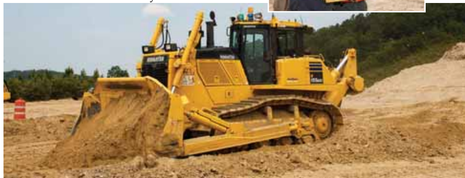
Attendees could operate all equipment, including the D155AXi-8 RC dozer, which is controlled remotely via a radio transmitter.
