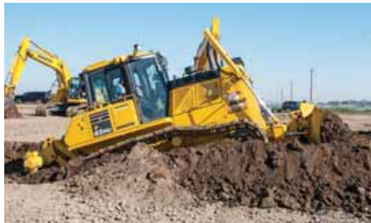
Customers help shape a reservoir with Komatsu intelligent Machine Control products, including this D65PXi-18 dozer.
