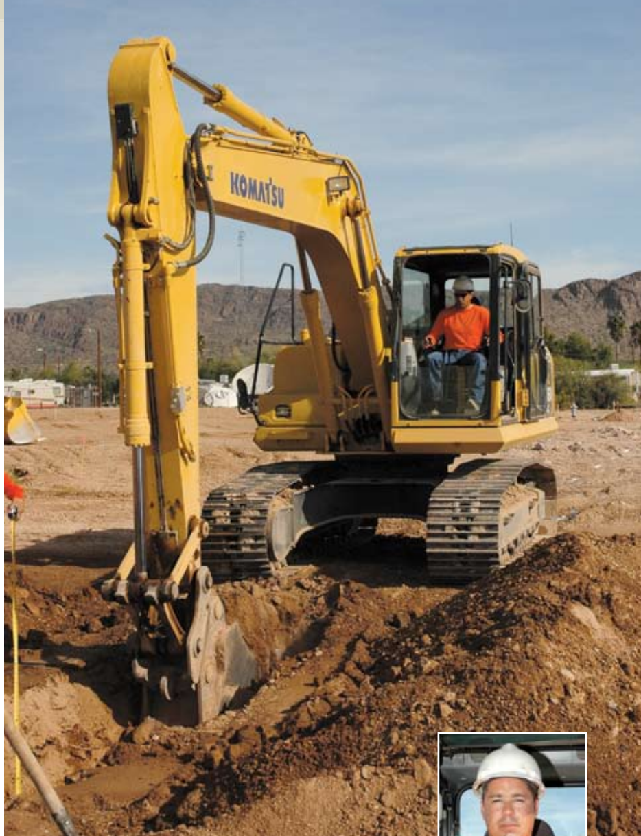
Superintendent Clay Jerald uses a Komatsu PC160LC-7 to dig a utility trench for a new development in Tucson. "It's smooth, quiet and easy to operate," Jerald said of the 36,740-pound machine.
